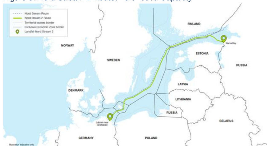
Figure 5: Nord Stream 2 Route, ~5.6 bcf/d Capacity
